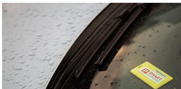
Figure 2-5 Smart Parking RFID Tag (source: Smart Parking)
